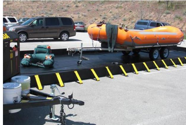
The TRV-3500 trailer is made of extra-rugged 2-by-4 inch, 10-gauge formed channel. The wheel and axle assembly feature leaf-spring suspension of up to 3,500 lbs. and 15-inch, white rimmed wheels. A powder-coated epoxy finish gives the entire package added weather protection.
